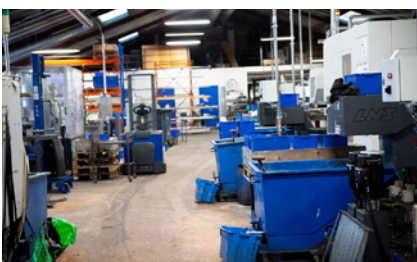
The turning department at Brandt Metal Industry with the central filtration system.
