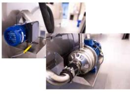
✓ 100 % stainless steel construction Produced with a stainless steel cabinet, tank cover, electrical cabinet, pumps and heating elements.
